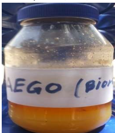
Plate 6. Sample of Bioresin from ground nut oil
