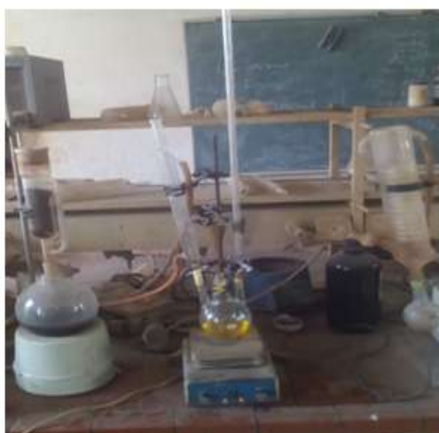
Plate 3. Epoxidation reaction set up
