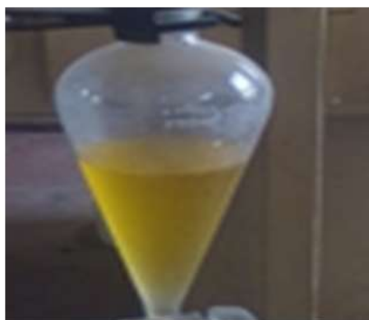
Plate 4. Sample of EGO produced from epoxidation reaction
