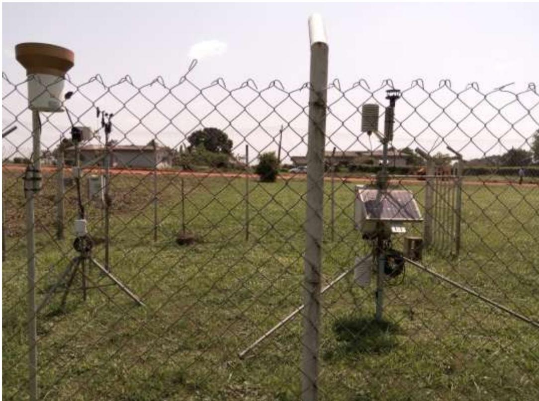
Figure 3.2: Experiment set-up of tipping bucket rain gauge at Site C.
