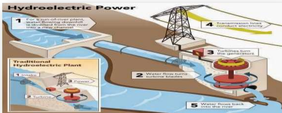
Figure (1): hydro dam electricity project.
