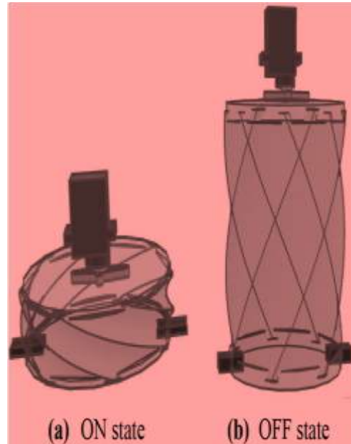
Fig. 3 Views of the ventilator in the ON (a) and OFF (b) states
