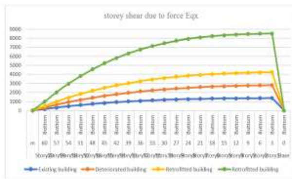
Graph 3.41 Storey shear due to force EQx
