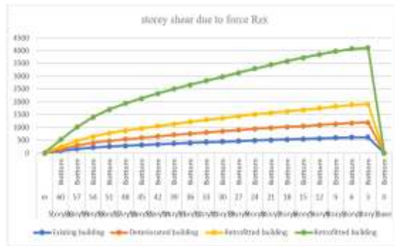
Graph 3.51 Storey shear due to force RSx
