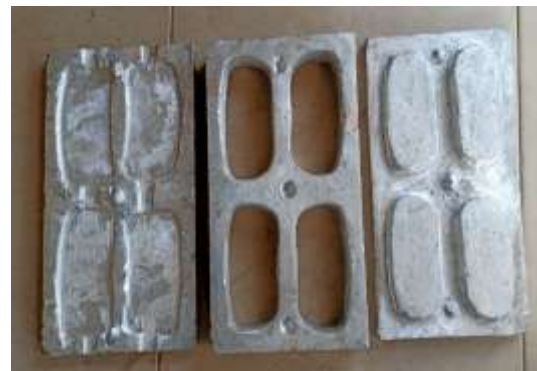
Plate 3: The fabricated Aluminium mould Source: Author Field Work, 2023
