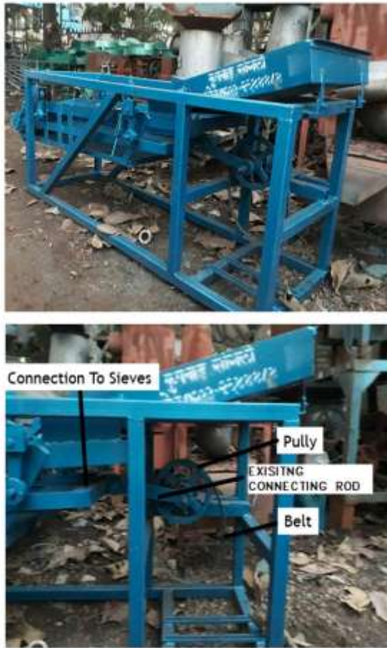
Fig -1: Existing Sorting Platform
