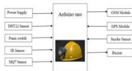
Block diagram of proposed system
