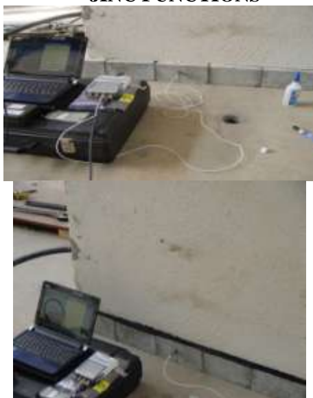
Figure 2. Experimental set-up used for the measurement of the wall transfer mobility [7]. a) First configuration: rigid connection between the wall and its support; b) Second configuration: Viscoelastic connection between the wall and its support.
