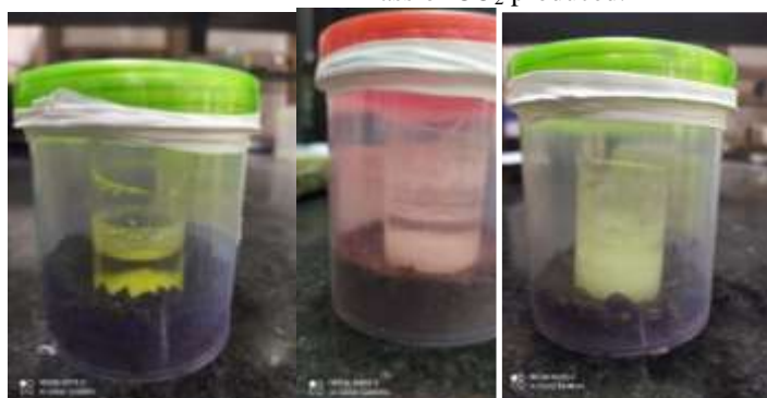
Only soil, Soil and polymer after 5 days, Soil and polymer after 25 days with KOH solution placed in it, and sealed respectively.
