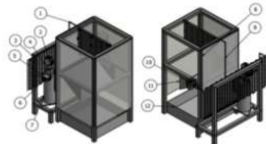
Figure 1. Schematic and position of the air-water harvester machine. 1. The condensing unit, 2. Pressure gauge outlet to compressor, 3. Condenser, 4. Compressor outlet pipe to condenser, 5. Pressure gauge inlet to compressor, 6. Inlet pipe to the compressor from the condensing unit, 7. Compressor, 8. Wall insulator, 9. Pipe from the condensing unit to the compressor, 10. Capillary pipe from the condenser to the condensing unit, 11. Where the dripping dew flows into the reservoir, 12. Reservoir.
