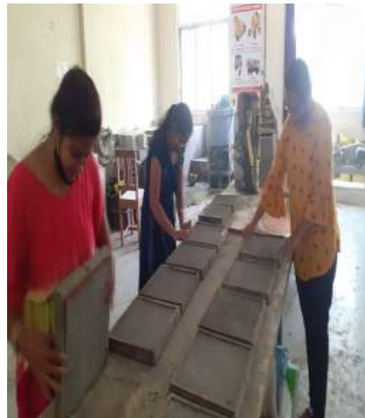
Figure 3. Casting of tiles
