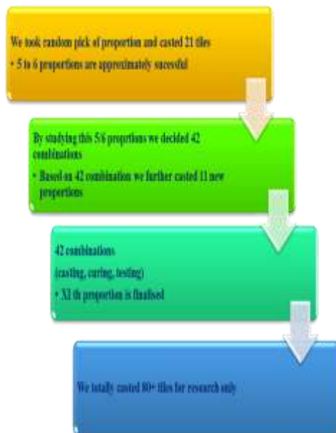
Figure 2. Flow of casting process of tile
