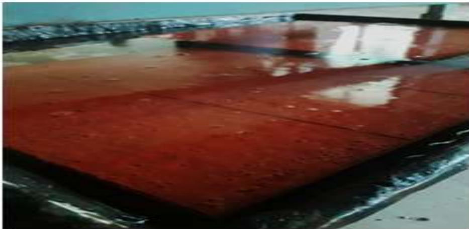
Figure 6. Water absorption test for tile
