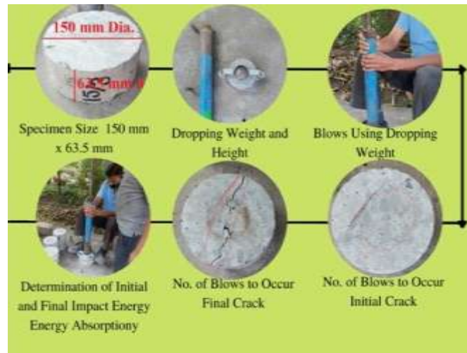
Fig. 8 Test Setup for Impact Resistance Test
