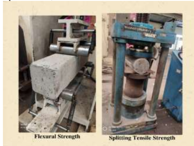
Fig. 5 Test Setup for Flexural and Splitting Tensile Strength
