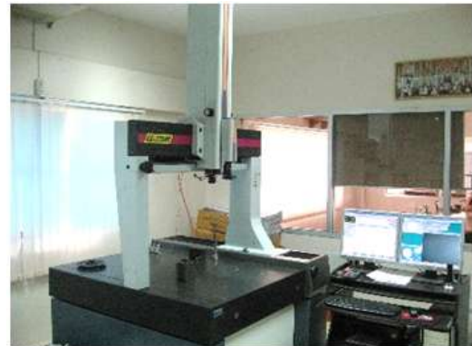
Fig 1.6 Shows a CMM machine for checking PCD distance in drilling and tapping.
