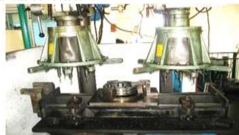
Fig 1.4 shows the installation of the fixtures with the drilling and tapping machines.
