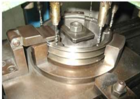
Fig 1.5 shows drilling and tapping using the created clamping device.
