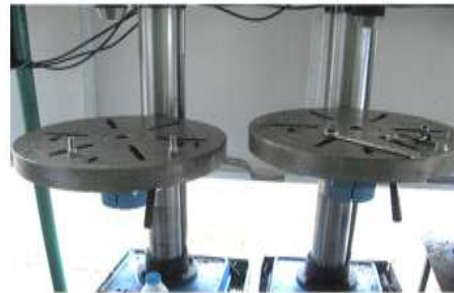
Fig 1.2 Shows the drilling and tapping machine before installing the clamping device.
