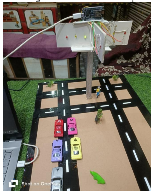
Fig. 1. Physical prototype intersection with LED traffic signals and controller mounted on pole
