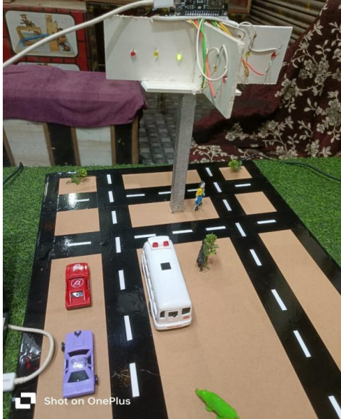
Fig. 2. Prototype traffic layout including an ambulance vehicle for emergency priority testing
