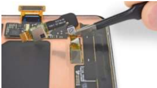
Fig 2: Hardware component Ultrasonic Fingerprint Scanner
