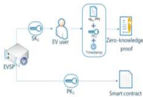
Fig 4. Step 1: EVSP distributes (SKC , PKC) and creates smart contract. Furthermore, the user creates a zeroknowledge proof for subsequent verification.
