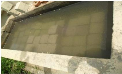
Figure 3.3 Normal water curing
