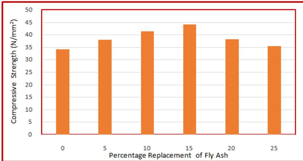
**Figure 4.2 – Compressive Strength of SWC Samples**
