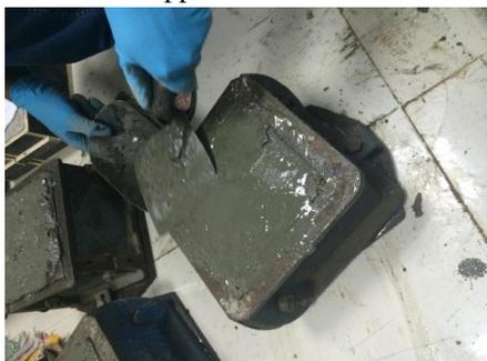
Figure 3.1 Samples levelled using Trowel
