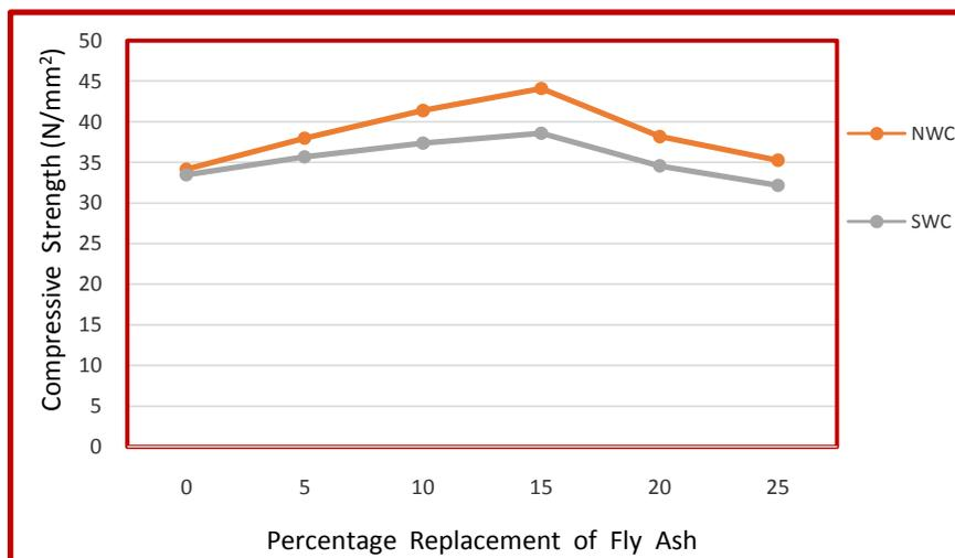
**Figure 4.3 – Compressive Strength of Normal Water and Sea Water Cured Samples**
