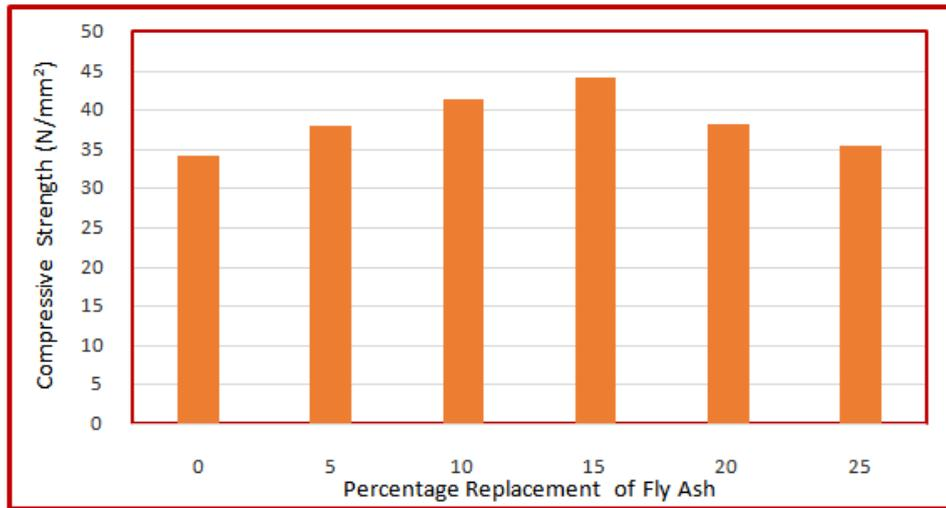
**Figure 4.1** – Compressive Strength of NWCSamples
