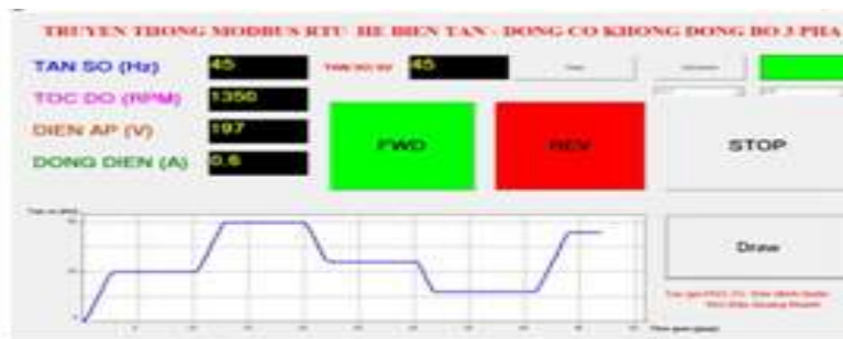
Figure 7. Modbus communication interface on PC for pairing with inverter
