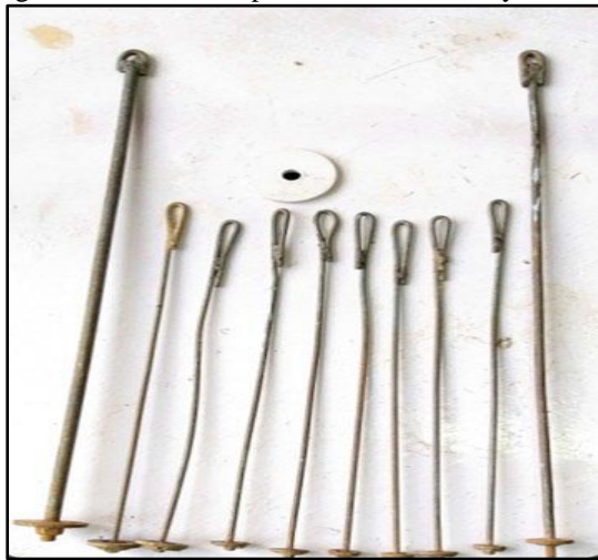
Fig. 14: Anchor piles used in laboratory tests
