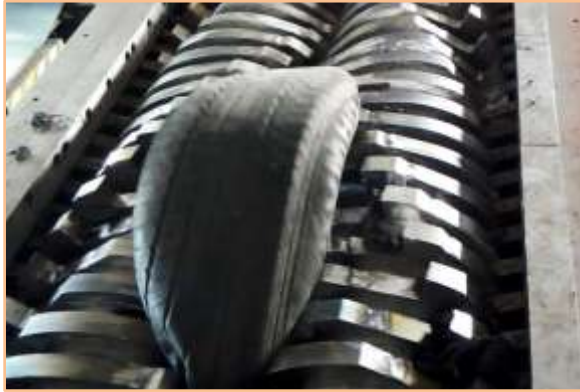
Fig – 2: Ambient Grinding of ELTs
