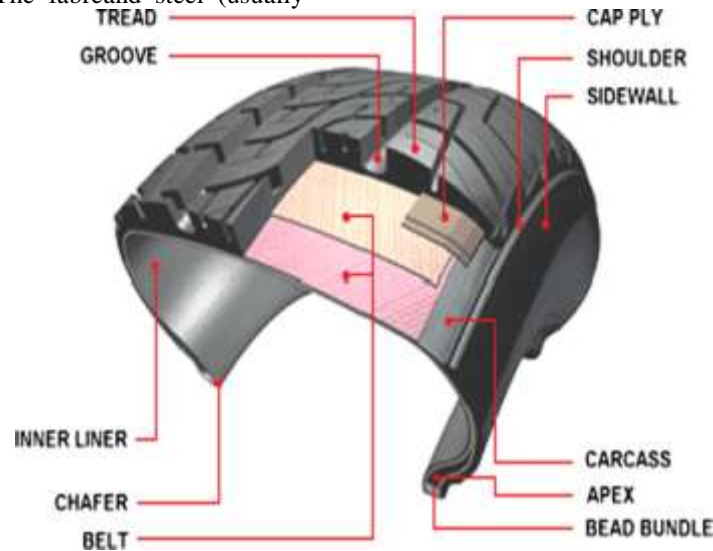
Fig -1: Tyre structure, adapted from [17]
