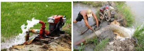
Figure 1: Using a diesel engine to pump water from a well and ditch.
