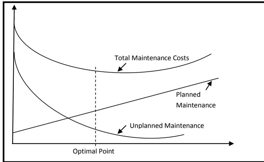
Figure 1: Trade-off between Planned and Unplanned Maintenance.
