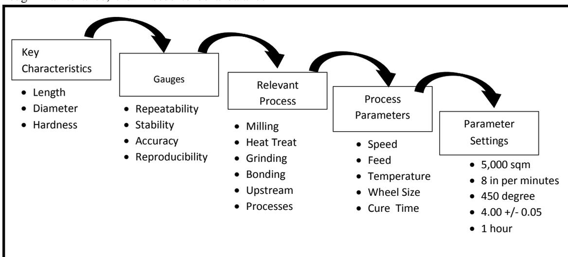
Figure 2: Key Characteristic to Process Parameters
