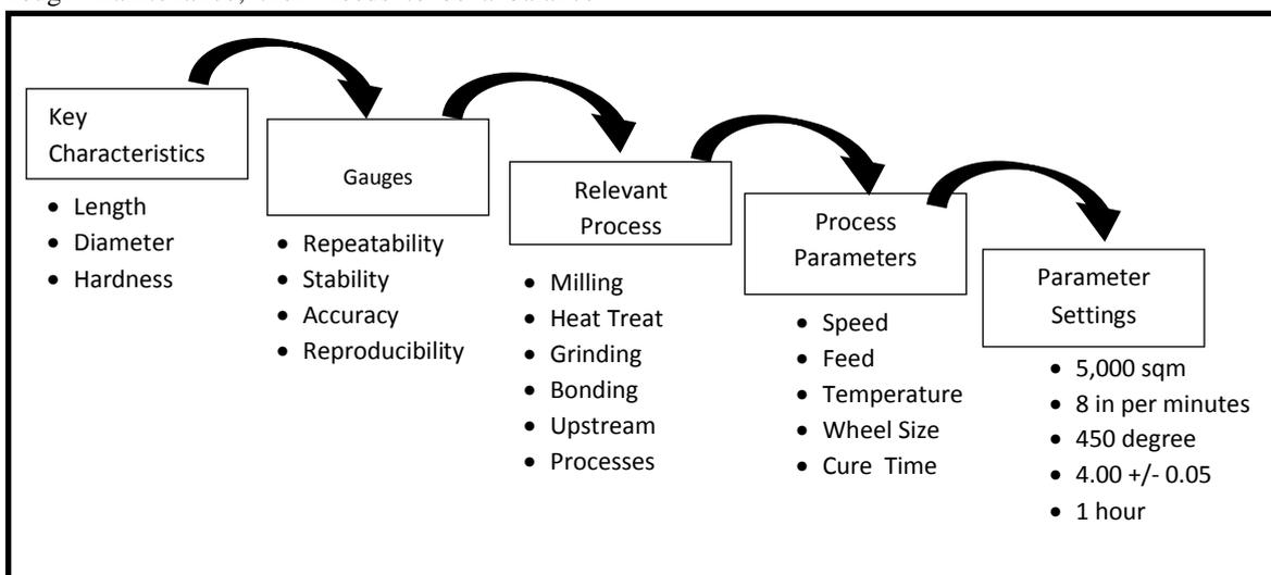
Figure 2: Key Characteristic to Process Parameters
