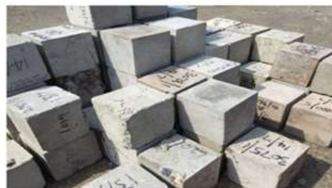
Curing of specimens
