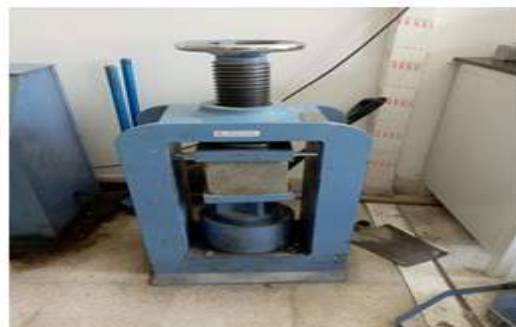
Fig.4.7 Compression Testing Setup
