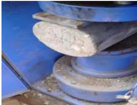
Fig.4.9 Split tensile Testing Setup
