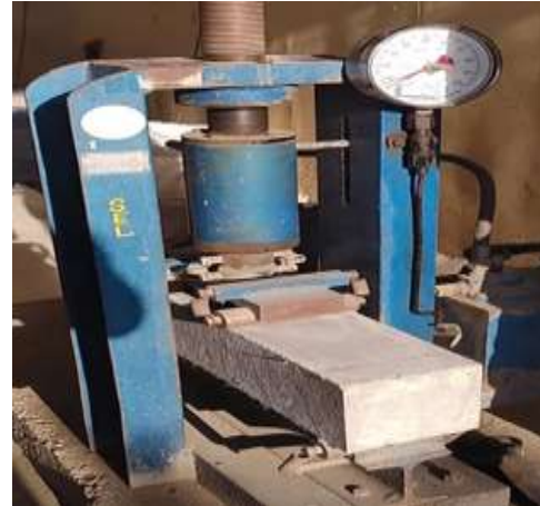
Fig.4.11 Flexural Testing Setup
