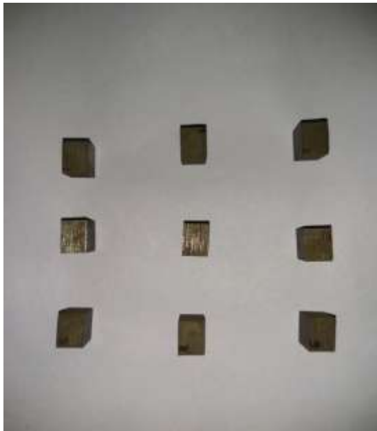
Figure 10 Specimen of size 10x10x6 mm after WEDM
