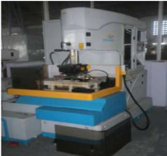
Figure 2 Experimental setup of WEDM
