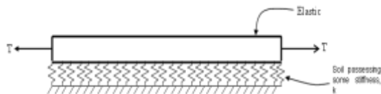
Figure 2.2 Illustration of the assumption of various methods for providing for interaction among the foundation plate spring elements
