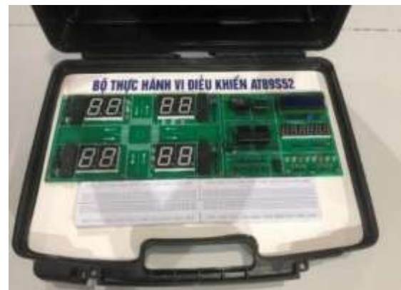
Figure 12: Complete model fabrication of Traffic light signal system using Master and 4 Slave microcontroller network
