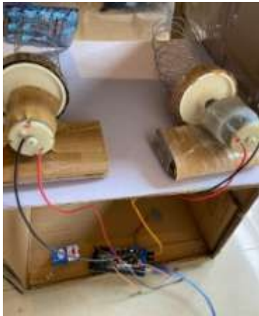
The machine's internal structure includes DC motors, an Arduino mega, and spirals.
