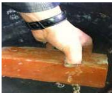
Figure 3.3 Water absorption test on bricks
