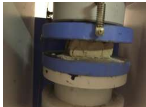
Fig 3.1 Compression testing on mycelium brick
