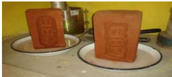
Figure 3.2 Efflorescence test on bricks
