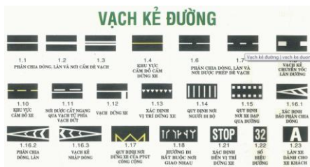
Road markings comply with QCVN 41:2012
