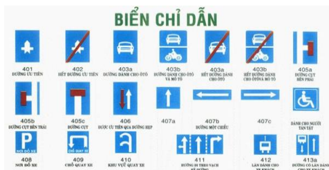
Additional signage according to Vietnam road regulations
