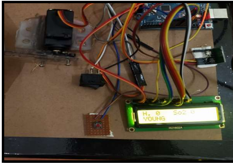
Figure 3: Young Mode, The frequency of pumping in this mode is changed from child mode and is set in accordance with the breathing pattern of adults.
