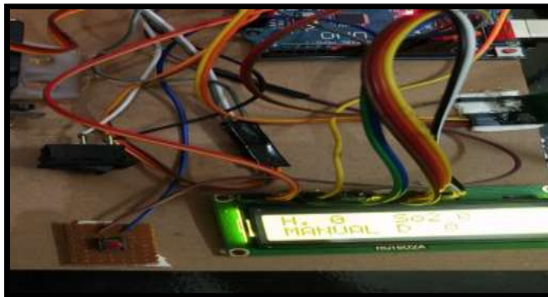
Figure 4: Manual Mode, As in many cases it has been observed that different patient require different speed at which air is being pumped. This situation could easily be tackled by using this mode. After the adult mode when switch is long pressed the device gets activated into the manual mode and this is shown on the display itself. Manual mode allows the user to adjust the frequency of pumping according to the patient.
