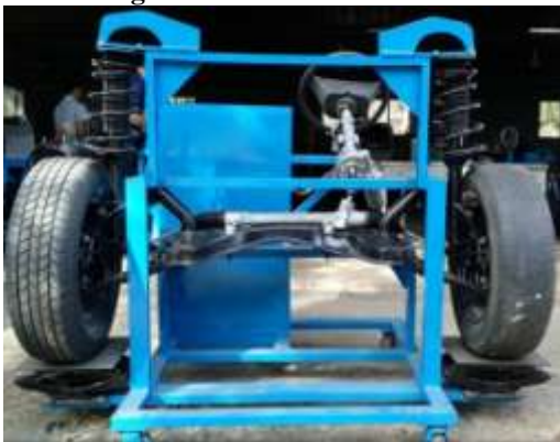
Fig.7. Semi-empirical model of electric power steering (EPS)
