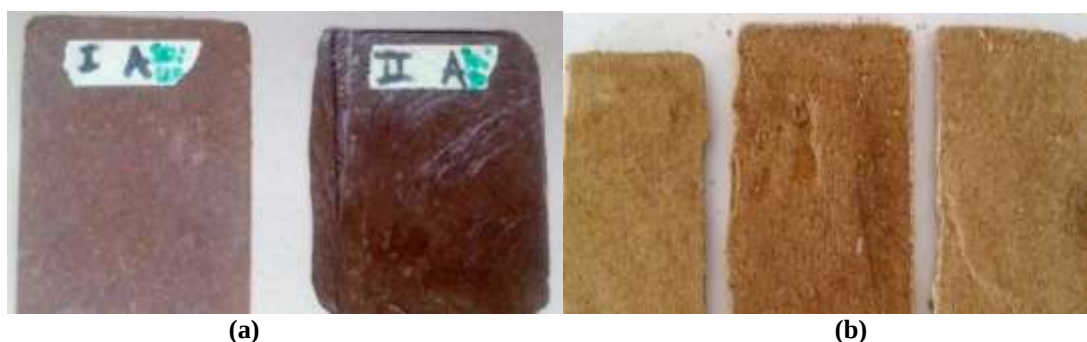
Plate 1: (a) Photograph of Hybrid Matrix from CissusPopulnea Bark Powder and Epoxy Resin (b) Photograph of Hybrid Matrix from Cissus Populnea Bark Powder and Hardener
