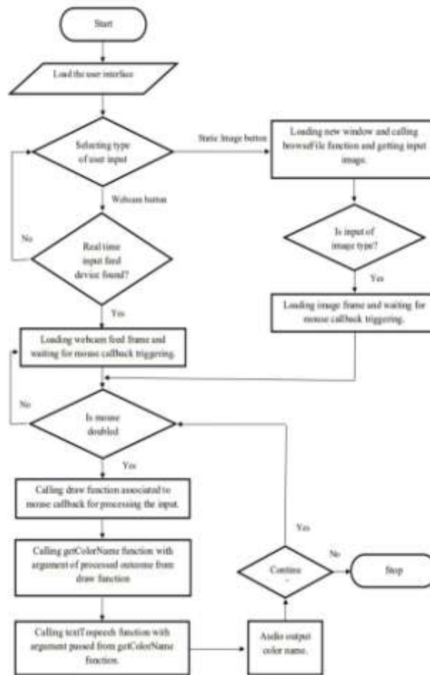
Figure 1: Flowchart for Workflow of Colour Detection from Image
