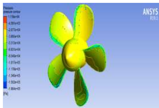
Figure 25: Pressure contour on the propeller at 200 rpm
