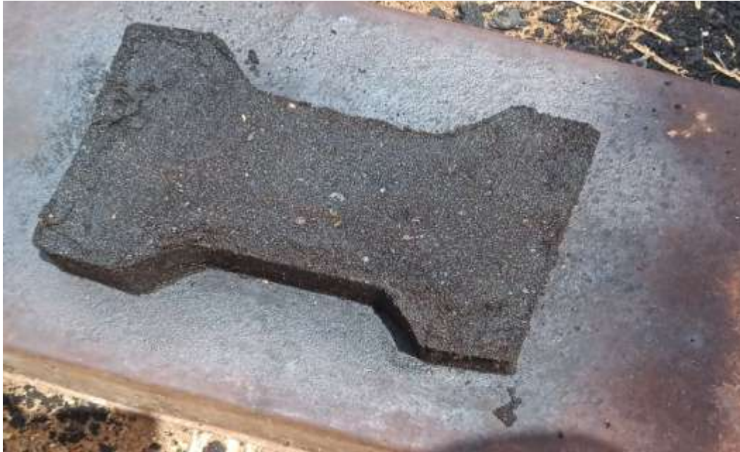
Plate 2 Casting and Drying of waste nylon interlock
