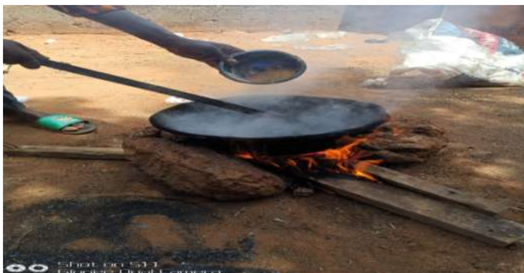
Plate 1 Heating waste Nylon and Adding sand
