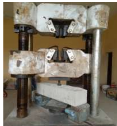
Figure 4: Beam set-up on a universal testing machine
