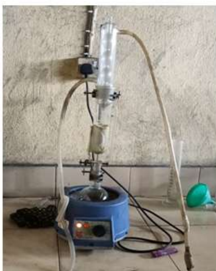
Figure 2: Illustration of the apparatus for Soxhlet extraction
