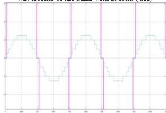
Figure 8: The zoomed view of output current waveform of the MLI with R-Load (GA)
