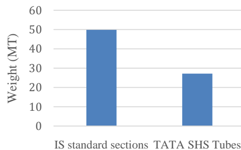
Graph 7 – Weight of bracings for different steel sections.
