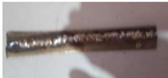
Plate 1: Rear view of the specimen (Austenitic stainless steel)
