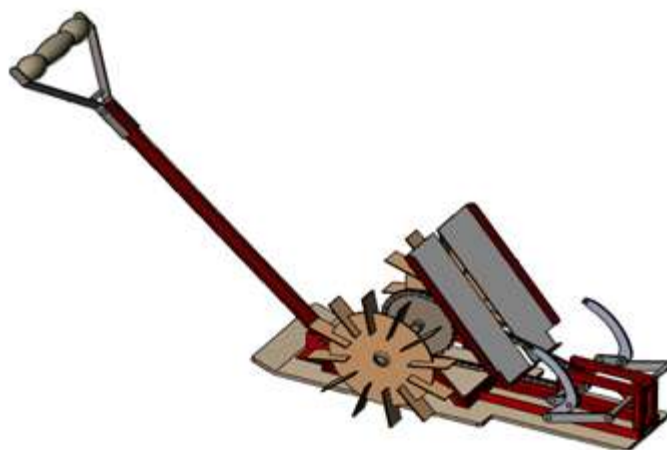
Fig. 2. Isometric Drawing of the Designed Manually Operated Rice Transplanter
