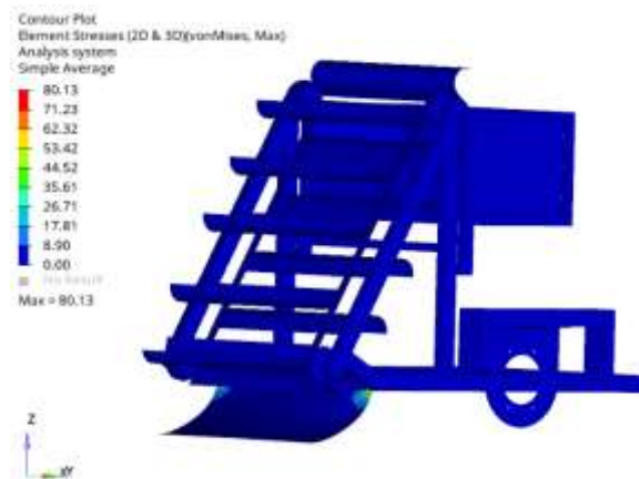
Figure 3 – Stress Analysis of Design 1
