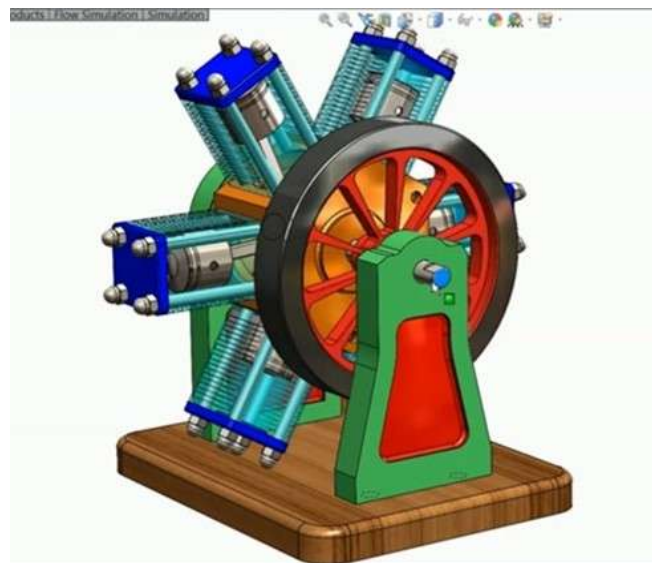
Figure 3.1: Final assembly of Radial engine
