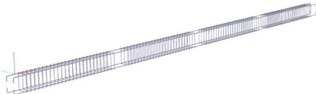
Rebar Cage view of Beam
