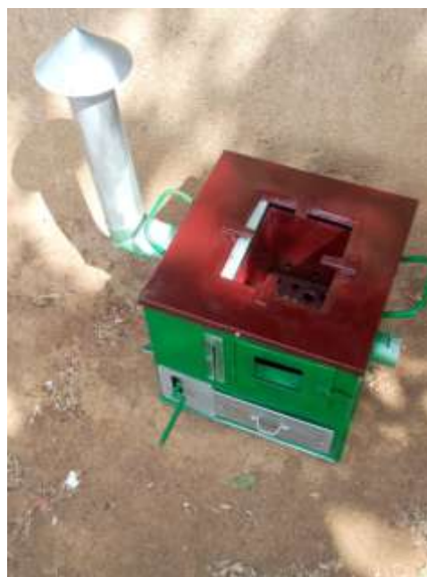
Plate 4: Complete fabrication of the briquette-fired adjustable stove
