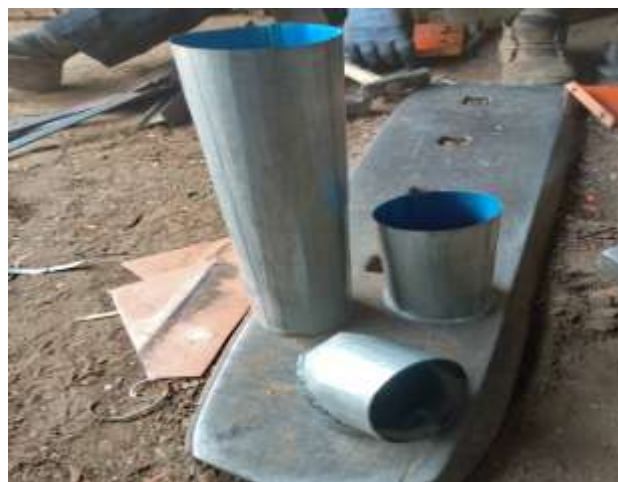
Plate 3: Shows the chimney pipe.
