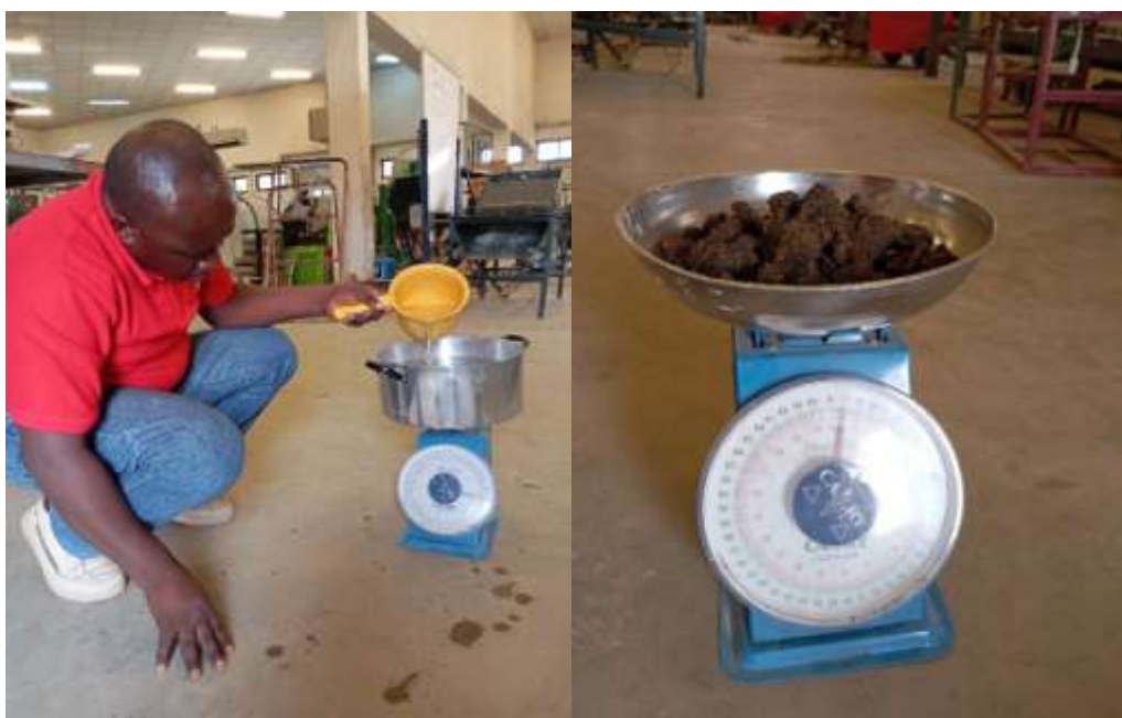
Plate 5: Measuring the mass of water and fuel during performance evaluation.
