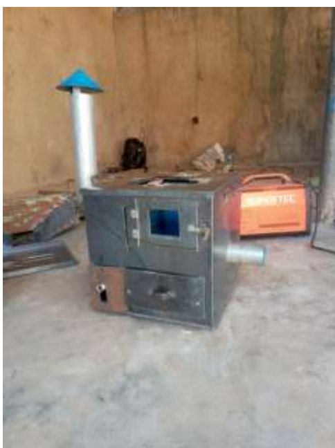
Plate 4: Complete fabrication of the briquette-fired adjustable stove
