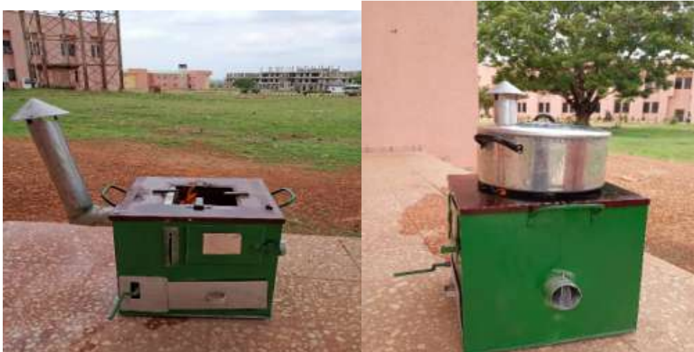
Plate 6: Experimental Set-up for Water Boiling Test
