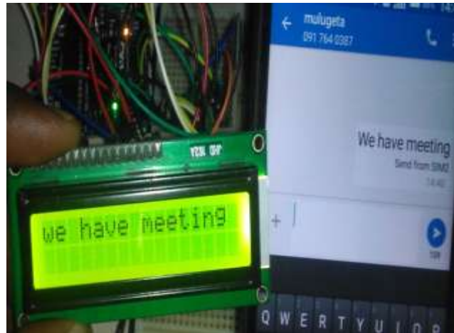
Figure 6. Received and Sent Message Using Bluetooth Module Display System.
