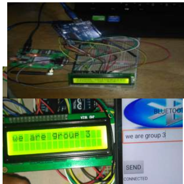
Figure 7. Default Message on LCD (top) and Received and Transmitted Message (bottom).
