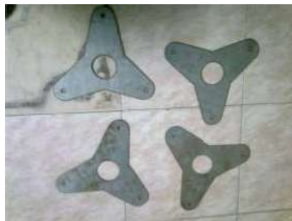
Fig9 Plasma Arc cut Tri-Star wheel web
