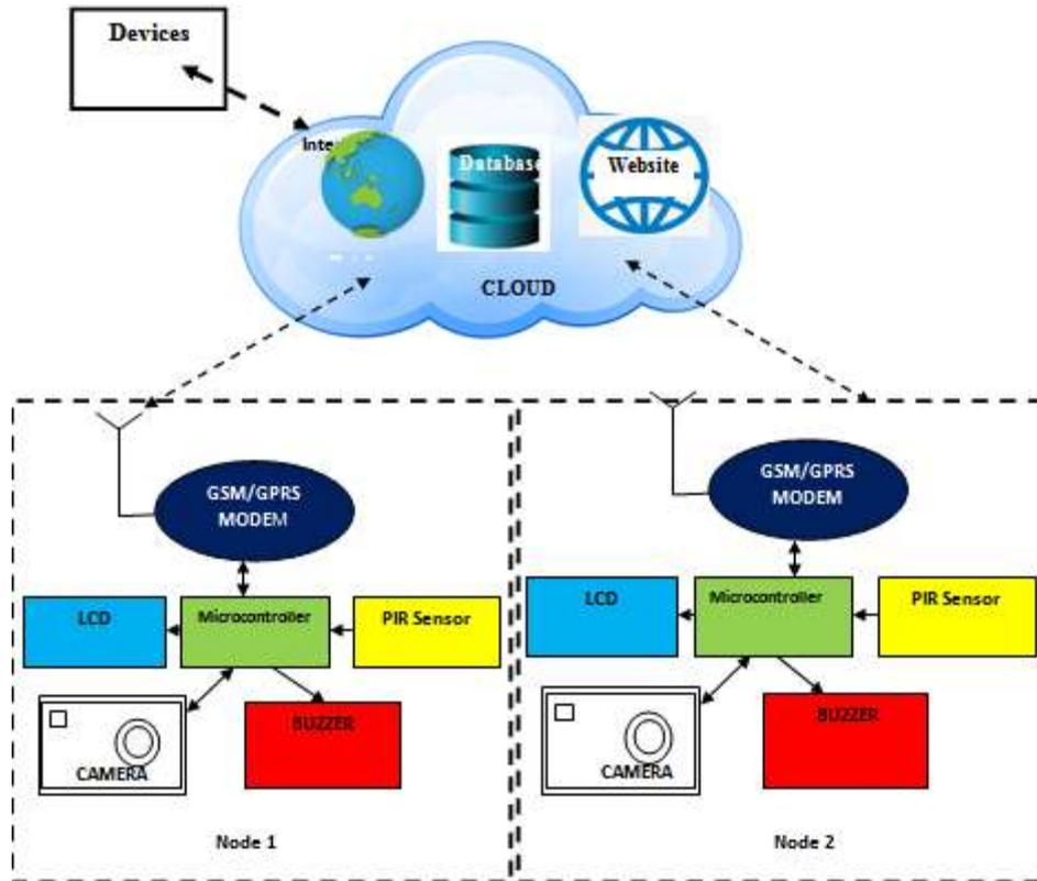
Figure 1: Block Diagram of the Intruder Detection System
