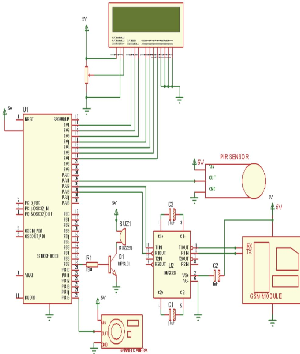
Figure 4: Schematic Diagram of the Intruder Detection System
